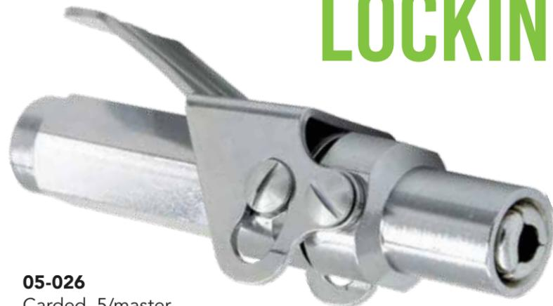
The quick connect coupler easily attaches and disconnects from fittings with one simple motion. The coupler conveniently swivels 360° for access to any fitting location. Solid steel construction allows the coupler to build up to 8,000 PSI and still disconnect with ease. 1/8" NPT.
