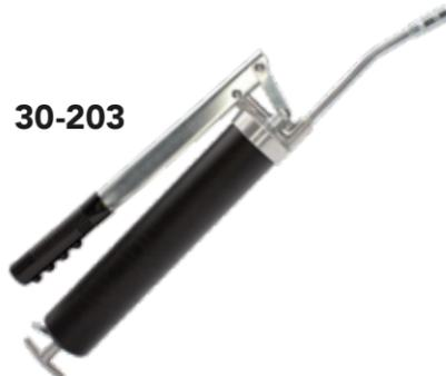
An improvement of the 30-200, this gun has a textured barrel and rubber handle grip for added ease of use. 2-way loading: 14 oz. cartridge or suction load. Includes 5-3/8" angled pipe and coupler. Added bleeder valve and locking plunger provide for easier priming. Develops up to 6,000 PSI. Delivers 1 oz./40 strokes.
